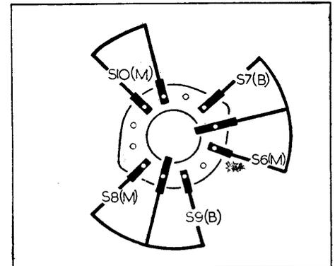
Diagram of the mains/battery switch unit.
