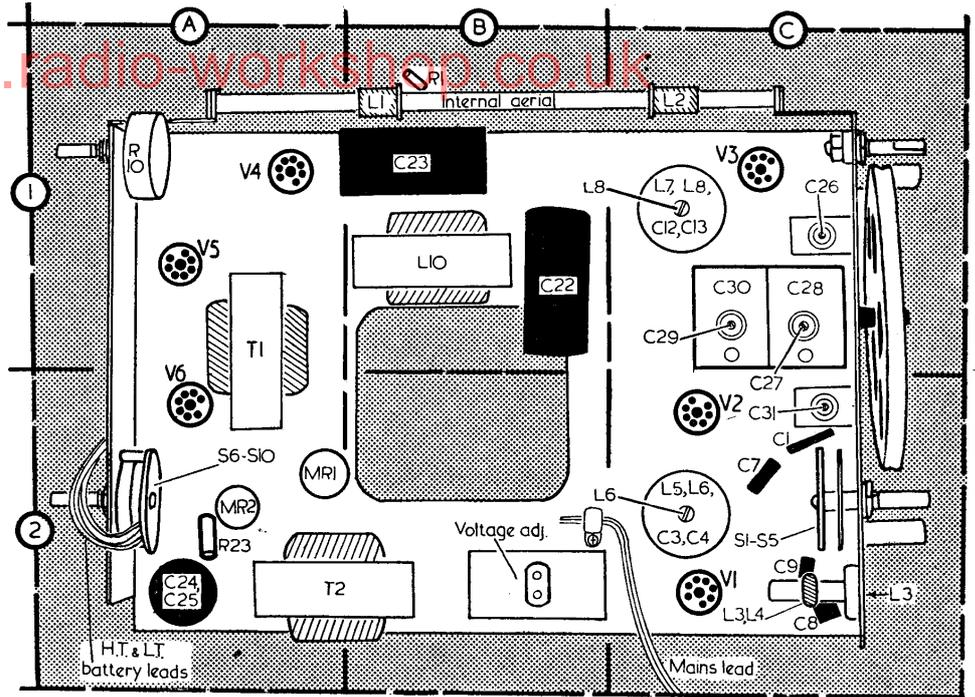
Rear illustration of the chassis. The waveband switch unit **S1-S5** and the mains/battery switch unit **S6-S10** are identified. These units are shown in detail in col. 3.
