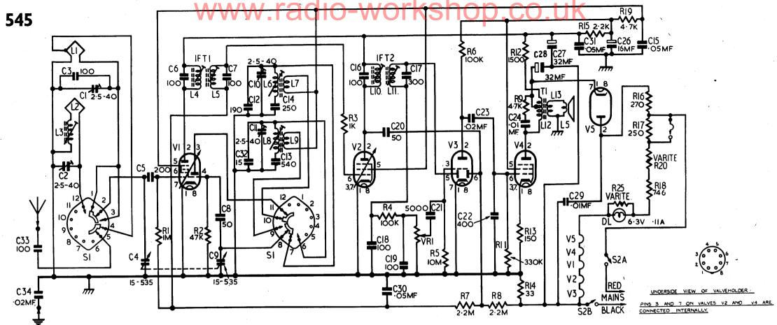
Note—SI is viewed from knob end of switch-RI6, RI7 and RI8 are one unit Part No. 07/18831-C27 and C28 are one unit Part No. 07/99174.
