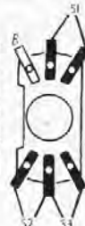
Diagram of the waveband switch unit, drawn as seen from the rear of an inverted chassis.
