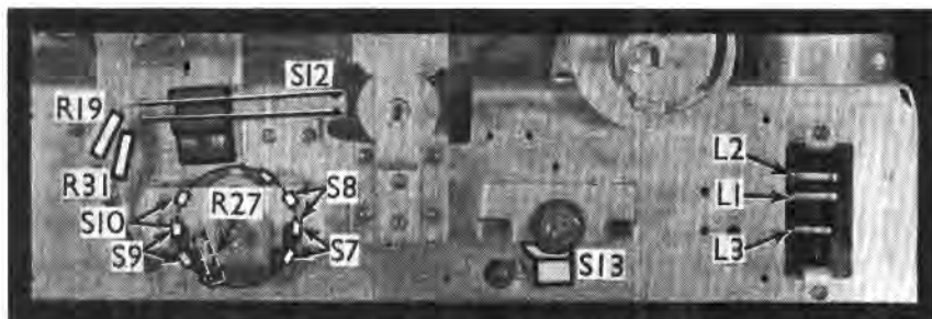
Front view of the lower part of the chassis, showing the tone control, muting and quiet tuning switches.
