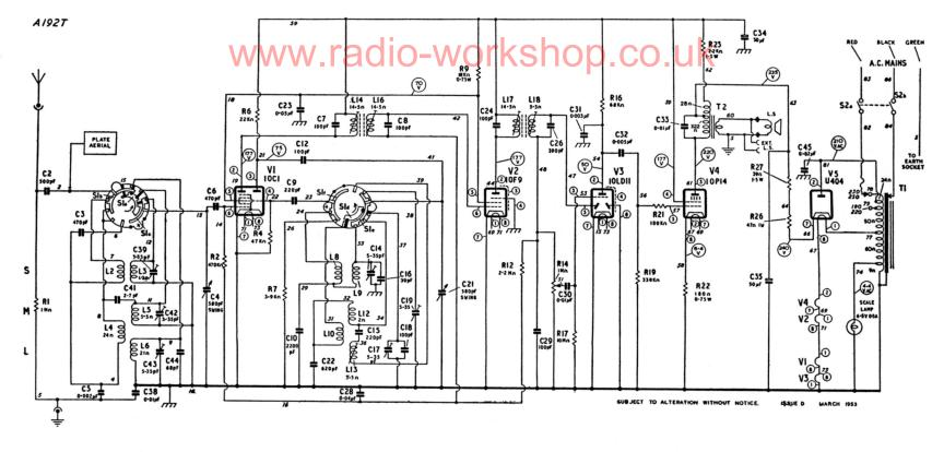
The switch wafers are drawn as seen from the rear of the receiver, and the lugs marked with a cross are the nearer to the chassis. The black contacts and inner rotors are on the hidden sides of the wafers. Blank contacts and anchoring tags are shown by a spot.
