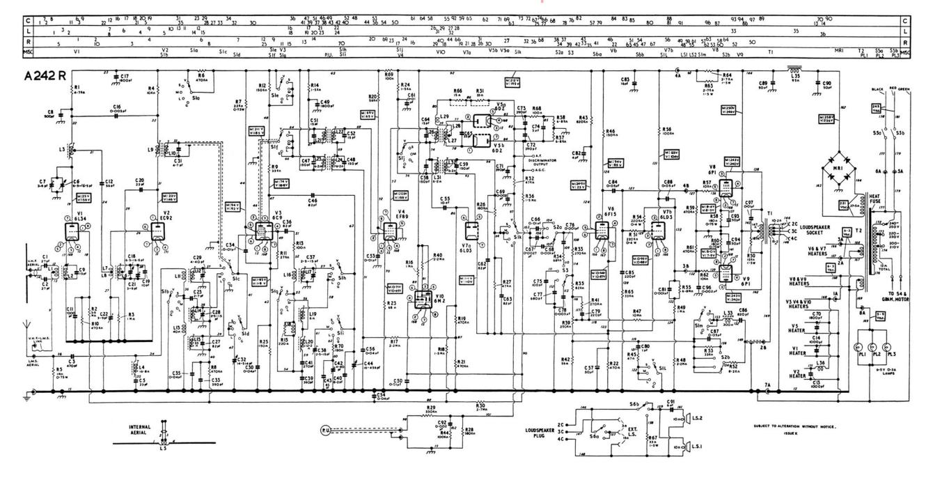
The Wave-band switch (S1a-S1m) is shown in the Band II position while the Bass (S2a-S2b) and Treble (S3) tone switches are shown in their minimum response (4) positions respectively. The Loudspeaker switch (S6a-S6b) is shown in the Internal position.
