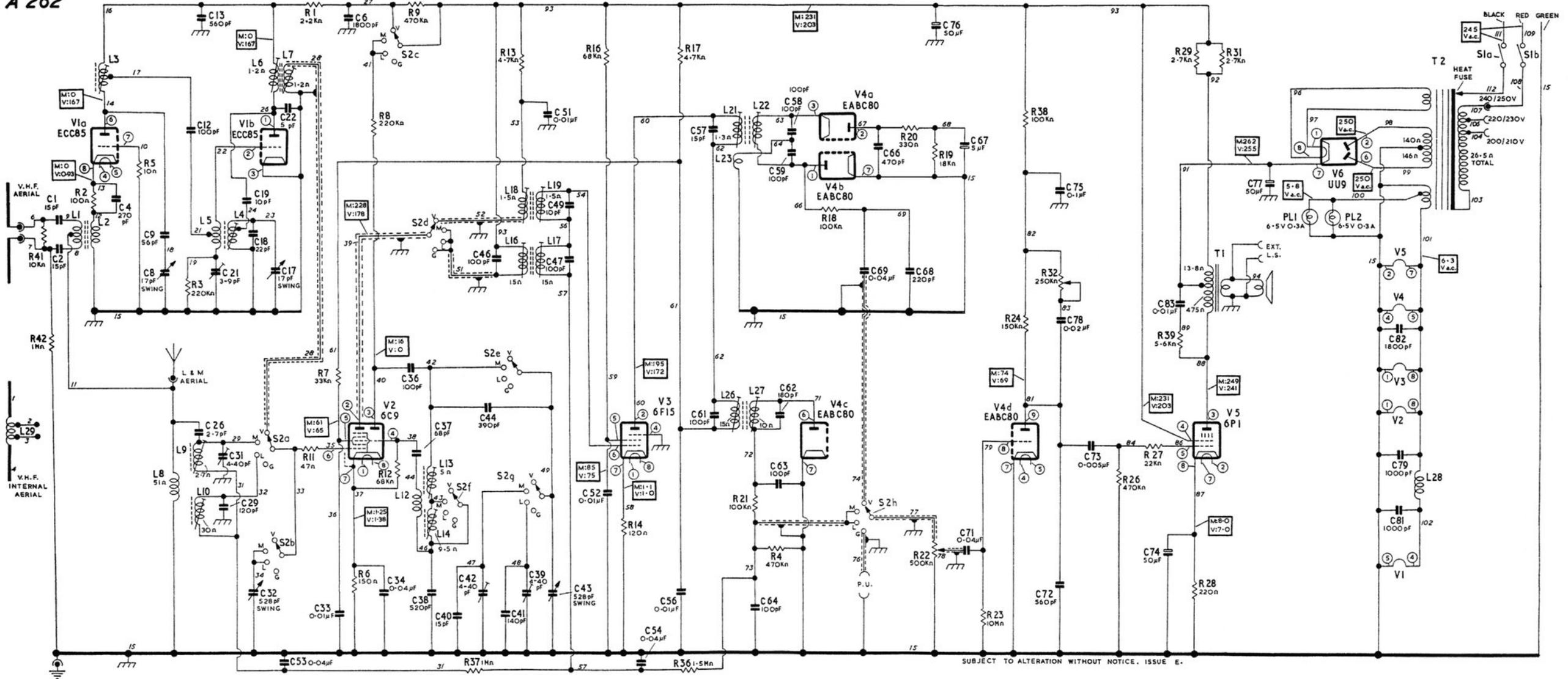
The wave-band switch (S2a-S2h) is shown in the L position.
