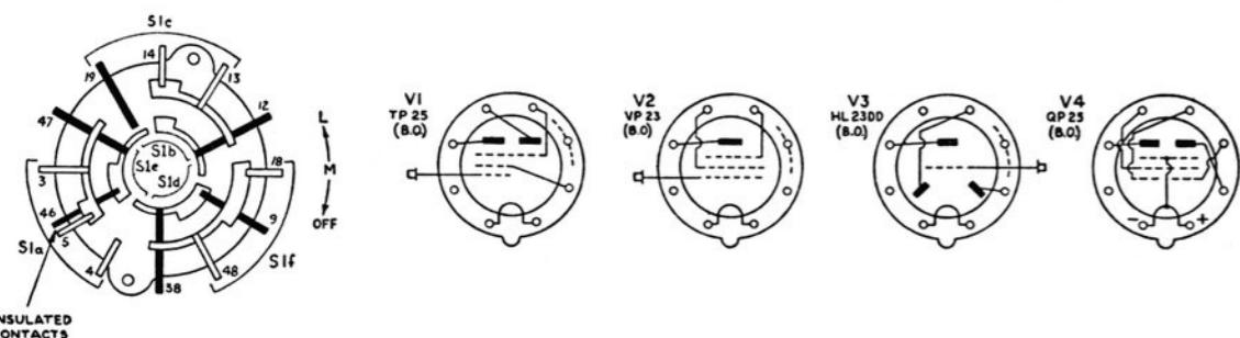
A 500 ohm/volt meter was used for taking the voltage readings; the receiver was switched to the medium wave band and operating under "no signal" conditions. In those cases where the resistance of a coil is omitted, the value is less than one ohm. The wave range switch is shown in the medium wave position. The switch wafer is viewed from the rear with the chassis upright, the black contacts and inner rotors being on the hidden side.
