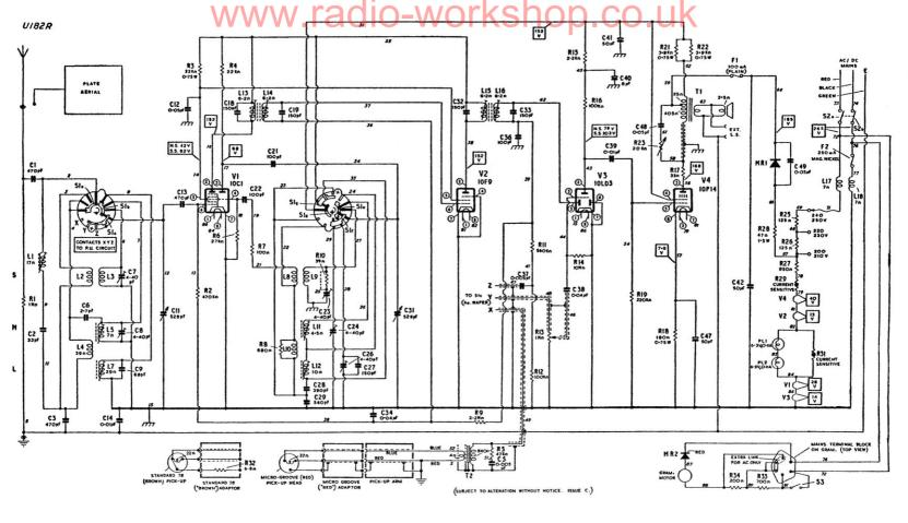
The wave band switch (S1a-S1g) is shown in the long wave position and is drawn as seen from the rear; rotate clockwise for medium, short, and gramophone. The black contacts and inner rotors are on the hidden sides of the wafers and the lugs marked with a cross are the nearer to the chassis. Blank positions and anchoring tags are shown by a spot.
