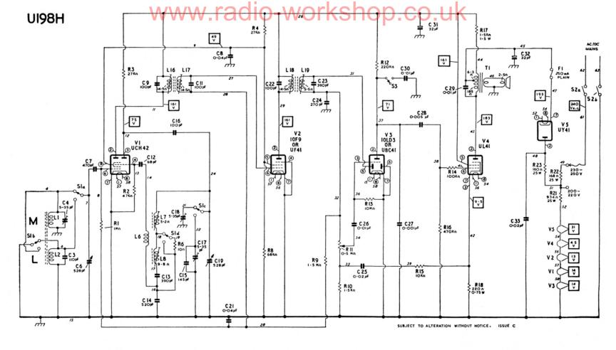
Circuit voltages are shown within rectangles and were measured with a 20,000  $\Omega/V$  meter while the receiver was switched to the M band under no-signal conditions.
