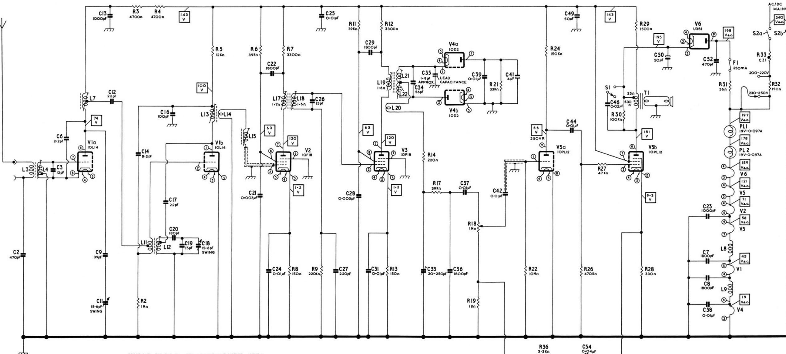
Circuit voltages are shown within rectangles and were measured with a 20,000 Ω/V meter under no-signal conditions.
