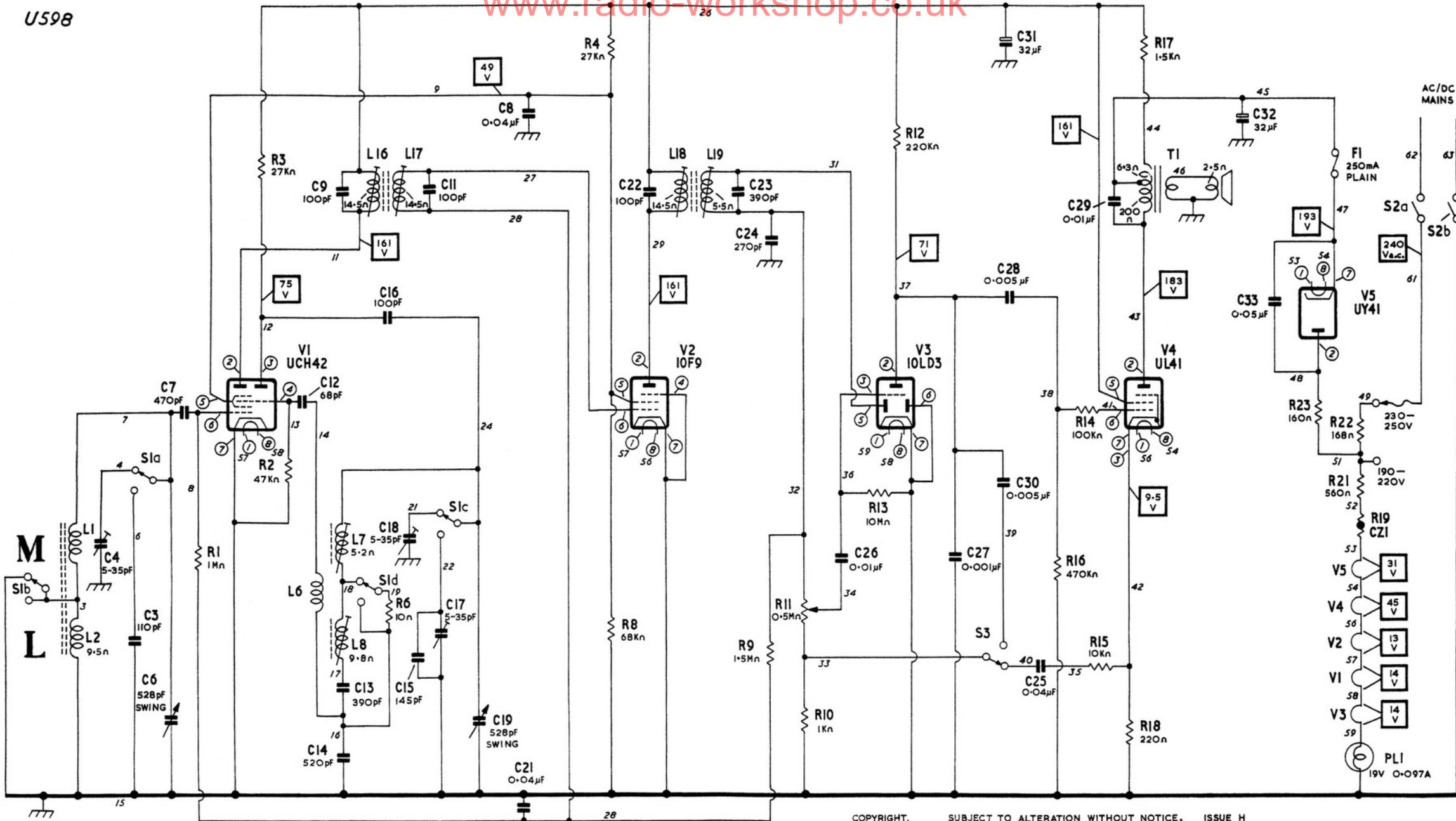
Circuit voltages are shown within rectangles and were measured with a 20,000 Ω/V meter while the receiver was switched to the M band under no-signal conditions. Where the resistance of a coil is less than one ohm the value is omitted.
