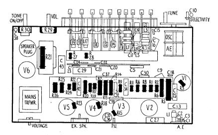
Coupling between V2 and V3, a doublediode triode, is by means of another permeability-tuned transformer, with tappings on both primary and secondary windings. Both the diodes of V3 are capacity connected to the transformer.
