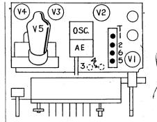
The trimmers for manually tuned circuits are indicated on this topof-chassis layout diagram. P.B. trimmers are paired near their buttons.
