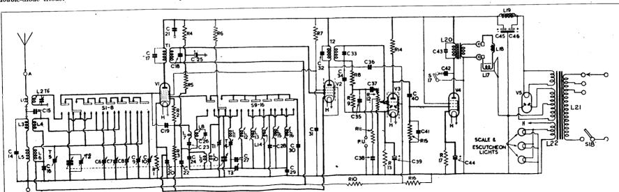
Preset capacities in the aerial stage and inductances in the oscillator stage are used for automatic tuning. The arrangement is straightforward on the whole and the identification of the trimmers assists recognition of the associated oscillator coils.
