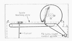
Sketch of the tuning drive cord system, drawn as seen from the front with the gang at minimum capacitance.
