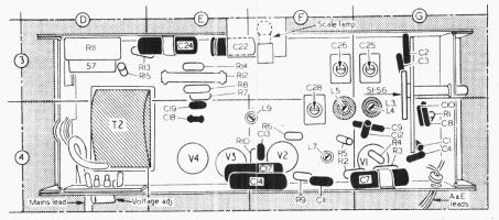
Underside view of the chassis, in which most of the alignment adjustments are indicated. A diagram of the S1-S6 switch unit is inset beneath the circuit diagram overleaf.
