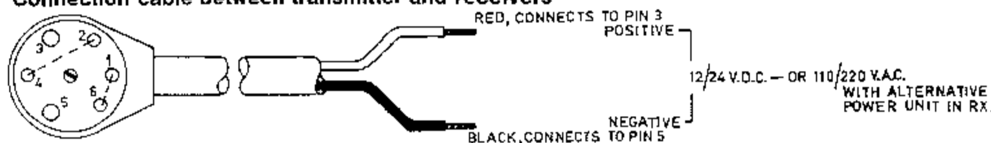
RECEIVER PLUG FEMALE HIRSCHMANN TYPE Mck 60z VIEWED ON PIN SIDE
